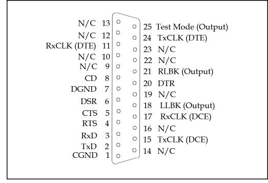
Figure 6 MPA-100 DTE Output Connector Configuration
